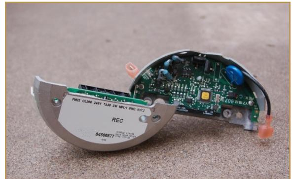
The introduction of an electronic module is an addition to the mechanical meter
