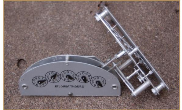
The electromechanical meter relies upon an intricate set of gears to accurately measure the amount of electricity used
