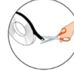
**3 CUTTING FOAM** - Cut long pieces of self-adhesive weather stripping material (foam, vinyl, etc.) for each side of the door jamb and door.
